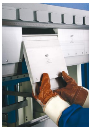
Simple insertion of upper tool from below without opening the safety latch.
